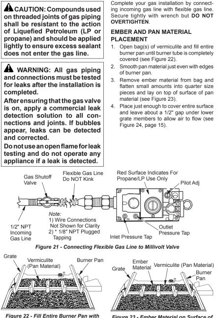
Figure 23 - Ember Material on Surface of Pan Material (Vermiculite)
